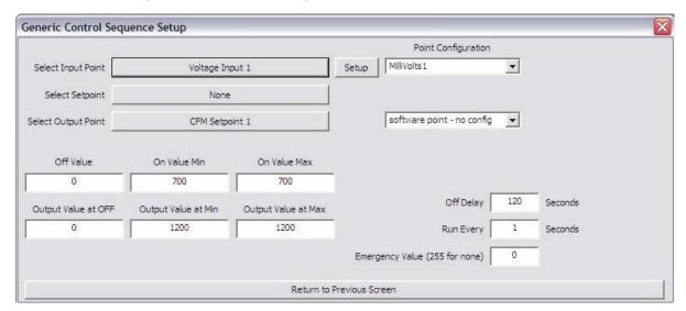
This time, the Input point is the same, but your Output is going to be CFM Setpoint. The limits will be the same, but the output will be whatever you want the CFM setpoint to be. I guess the same as the MAX Cooling CFM.
