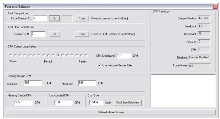
From this screen, you can test the operation of the damper alone and in relation to CFM Targets.
