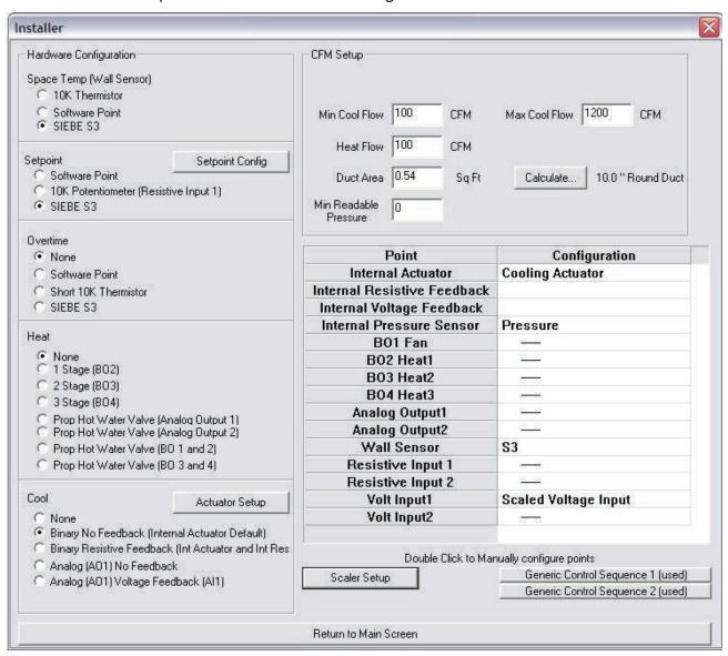
Here is an example how to setup a sequence where a CO2 sensor is used to set the CFM Setpoint to the Max CFM when CO2 level reaches a certain value.
